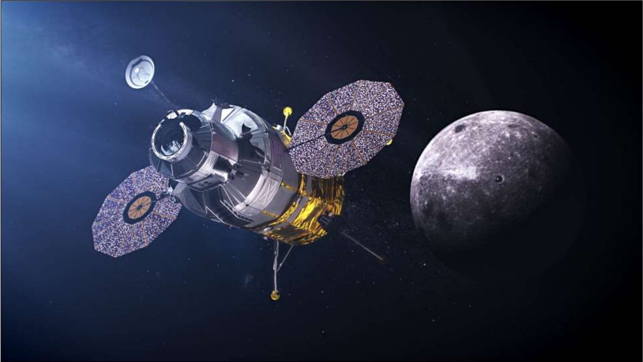
Figure 1: NASA's government concept for a Human Landing System includes an ascent, descent, and transfer module.
